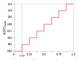
In consequence, the number of discrete values available, or "levels", is assumed to be a power of two. For example, an ADC with a resolution of 8 bits can encode an analog input to one in 256 different levels, since  $2^8 = 256$ . The values can represent the ranges from 0 to 255 i.e. unsigned integer or from -128 to 127 i.e. signed integer, depending on the application.
