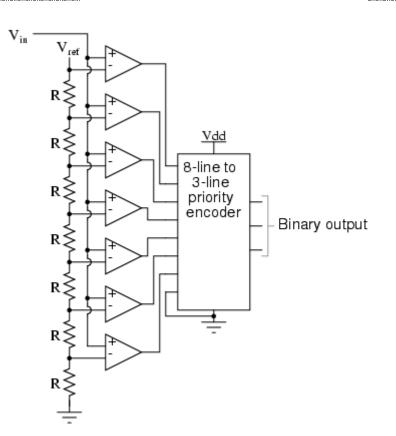
$V_{ref}$  is a stable reference voltage provided by a precision voltage regulator as part of the converter circuit, not shown in the schematic. As the analog input voltage exceeds the reference voltage at each comparator, the comparator outputs will sequentially saturate to a high state. The priority encoder generates a binary number based on the highest-order active input, ignoring all other active inputs.
