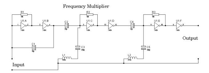
The filter used here is a band-rejection series LC type. Worse still, the rejection frequency is equal to the fundamental crystal frequency. The fundamental frequency is therefore attenuated, which is good. But the third harmonic is boosted by the smaller capacitor of 33 pF in combination with the inductor. Together they form the required band-pass filter. The same applies to the 12 pF capacitor in the next stage.
