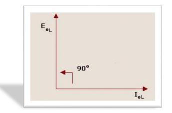
when used in conjunction with a resistive load bank, creates a lagging power factor load. Typically, the inductive load will be rated at a numeric value 75% that of the corresponding resistive load such that when applied together a resultant 0.8 power factor load is provided. That is to say, for each 100 kW of resistive load, 75 kVAr of inductive load is provided.
