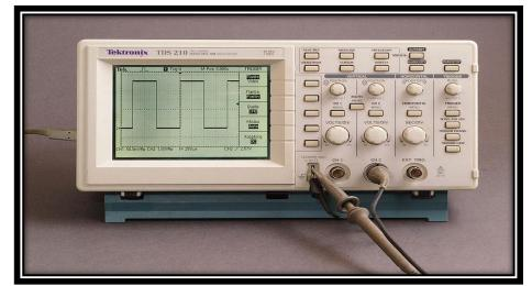
The principal advantage over analog storage is that the stored traces are as bright, as sharply defined, and written as quickly as non-stored traces. Traces can be stored indefinitely or written out to some external data storage device and reloaded. This allows, for example, comparison of an acquired trace from a system under test with a standard trace acquired from a knowngood system. Many models can display the waveform prior to the trigger signal.
