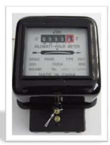
the meter move. The number of revolutions is recorded by the dials that you can see on the face of the meter. The speed of the revolutions depends on the
