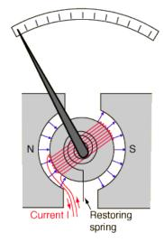
The most familiar use is as an analog measuring instrument, often called a meter. It is used to measure the direct current (flow of electric charge) through an electric circuit. The D'Arsonval/Weston form used today is constructed with a small pivoting coil of wire in the field of a permanent magnet. The coil is attached to a thin pointer that traverses a calibrated scale. A tiny torsion spring pulls the coil and pointer to the zero position.
