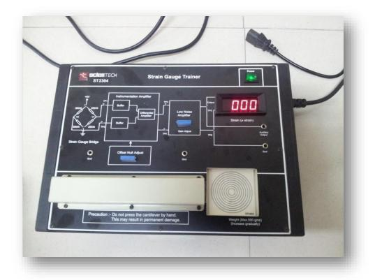
Therefore, the strain experienced by the test specimen is transferred directly to the strain gage, which responds with a linear change in electrical resistance.
