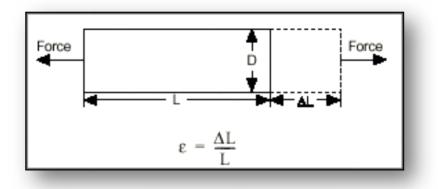
Strain can be positive (tensile) or negative (compressive). Although dimensionless, strain is sometimes expressed in units such as in./in. or mm/mm. In practice, the magnitude of measured strain is very small. Therefore, strain is often expressed as microstrain (me), which is e x  $10^{-6}$ .
