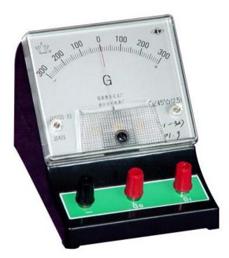
A galvanometer is a type of ammeter: an instrument for detecting and measuring electric current. It is an analog electromechanical transducer that produces a rotary deflection of some type of pointer in response to electric current flowing through its coil in a magnetic field.
