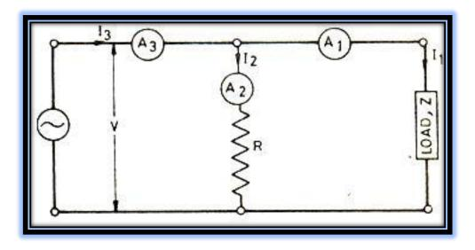
Three ammeters  $A_1$ ,  $A_2$  and  $A_3$  are connected in the circuit to measure currents flowing through the inductive circuit Z in which the power is to be determined, non-inductive resistance R and whole circuit respectively, as shown in fig.
