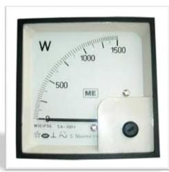
The traditional analog wattmeter is an <u>electrodynamic</u> instrument. The device consists of a pair of fixed <u>coils</u>, known as current coils, and a movable coil known as the potential coil.
