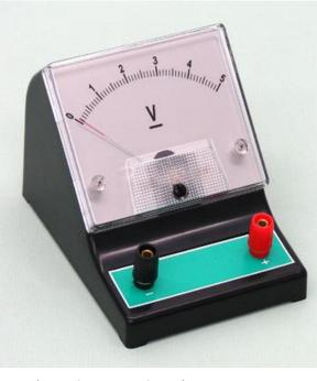
usually equipped to also measure current and resistance in the form of a multimeter, are standard test instruments used in electrical and electronics work. Any measurement that can be converted to a voltage can be displayed on a meter that is suitably calibrated; for example, pressure, temperature, flow or level in a chemical process plant.
