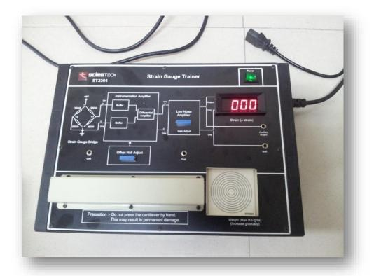
In summary, the ideal strain gage is small in size and mass, low in cost, easily attached, and highly sensitive to strain but insensitive to ambient or process temperature variations.
