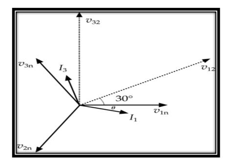
If the neutral point in a star-connected system is accessible, the power may be calculated from the readings of one wattmeter whose current coil has to carry the phase current and the voltage coil the phase voltage of the same phase. The total power is three times the power in one line.
