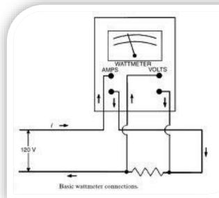
coil and considerable heat is generated. For higher voltages, the pressure coil circuit is designed for 110V, and a potential transformer is used to step down the voltage.
