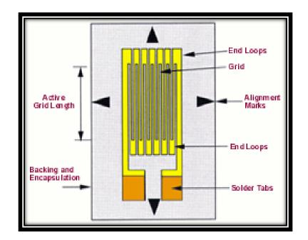
A fundamental parameter of the strain gage is its sensitivity to strain, expressed quantitatively as the gage factor GF. Gage factor is defined as the ratio of fractional change in electrical resistance to the fractional change in length:
